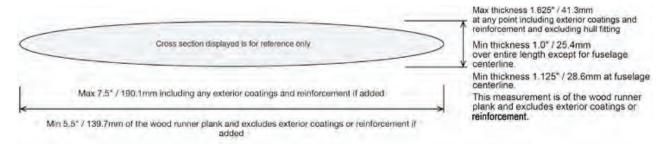
4.c Specifications B.3.a-f. Runner plank with exterior coatings and reinforcement where any exterior dimension is the minimum allowed (B.3.a-f) shall fail the minimum wood requirement
