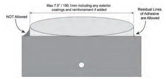
4.e Specification B.2.d, Crown: A 'fair continuous curve' may be one whose radius varies along its length. When not mounted on the fuselage and relaxed (under no load) the radius of the crown shall nowhere be concave, and no part of the curve shall be lower than the ends. The radius of curvature of the crown may vary along the length of the plank.
